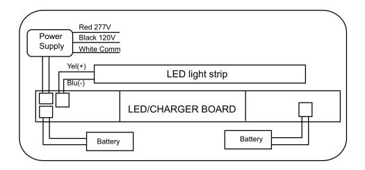
Note: Cap off the UNUSED input lead. Failure to do so can cause an unsafe operating condition.
